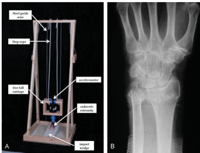
**Fig. 2** (A) FOOSH simulator device. (B) Experimentally created distal radius fracture.
